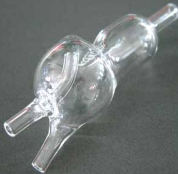
▲ Gas and Liquid Separator
