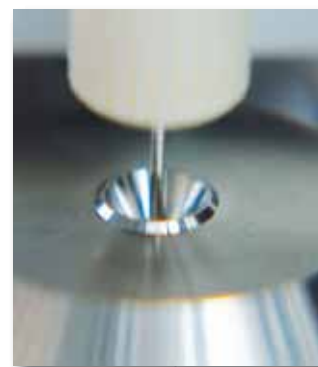
◀ Direct injection: Acidifying, purging, injecting
