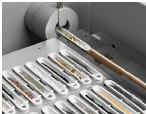
▼▲ Automatic solid sampler for 48 samples for the automated C, S, and Cl analysis as well as the automated determination of TOC and TIC.
