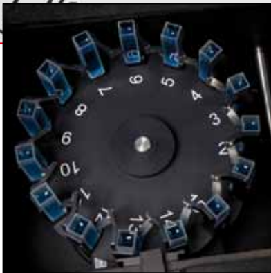
High sample throughput with the 15-cell changer or individual analysis with the single cell holder, the SPECORD® PLUS offers the ideal equipment for all requirements.
