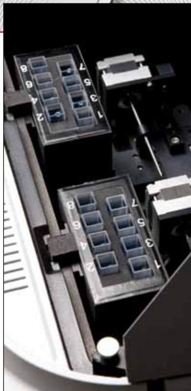
Sipper system for routine quantitative analysis
