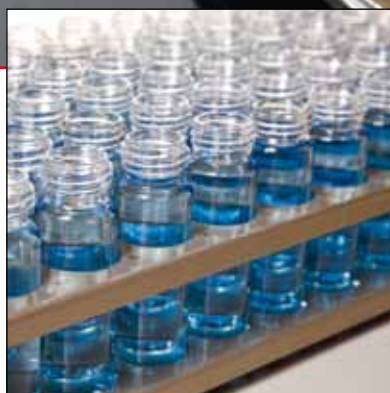
Autosampler for particularly high sample throughput
